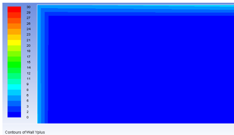
Fig. 3(e). Contour of Y+ on the base corner of the duct
