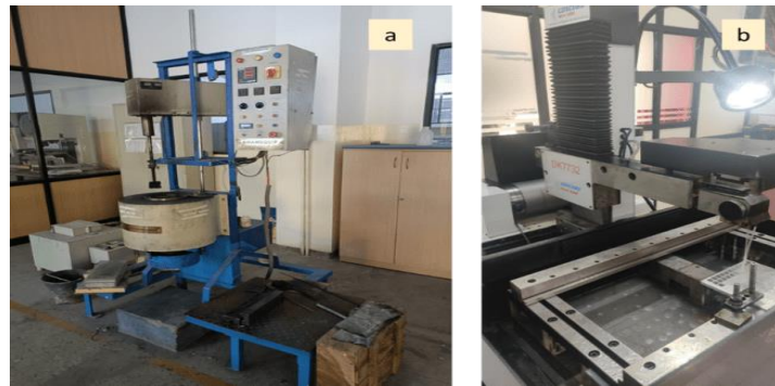
Fig. 2. Experimental Setup (a. Stir Casting for fabrication b. WEDM for Machining)
