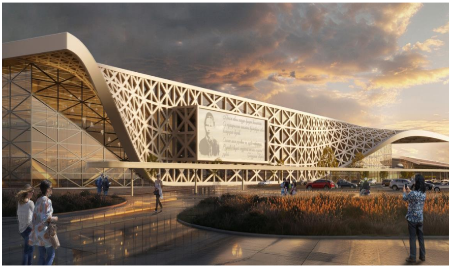
Fig. 3. The structure of the Kremlin wall is expressed through rhythmic vertical divisions, visually referencing the regular spacing of the fortification towers and battlements of the Kazan Kremlin, implemented using metal-ceramic panels (“QUANTUM CERAMIC”) and aluminum panels with an internal honeycomb core (“QUANTUM PARUS”)
