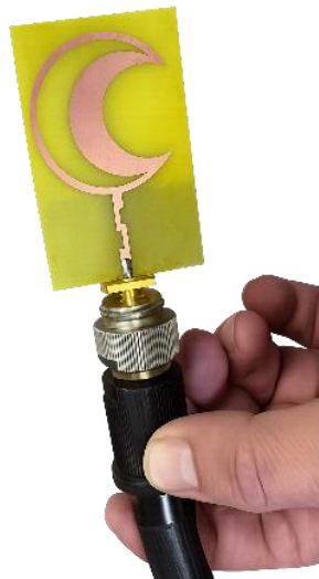
Fig. 9. Measurement setup: antenna connected to VNA via RF cable
