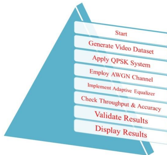
Fig 6. Demonstration flow chart of the proposed video broadcasting model using the QPSK Gaussian channel technique.
