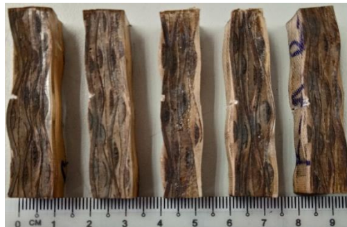
Fig. 1. Woven rattan fibre reinforced polymer before impact
