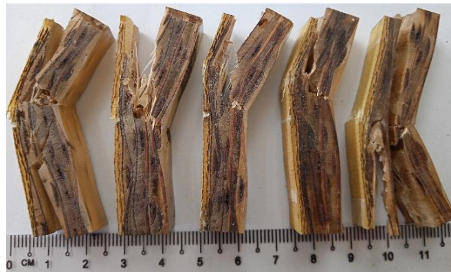
Fig. 2: Woven rattan composite after impact
