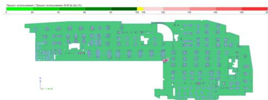
**Fig. 11.** Utilization factor for -2nd underground floor slab at elevation -6,200 for own weight and temperature actions, considering the specified reinforcement.
