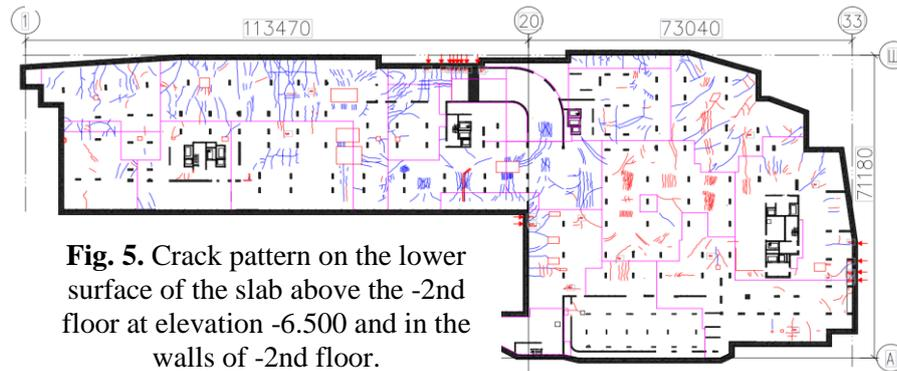
**Fig. 5.** Crack pattern on the lower surface of the slab above the -2nd floor at elevation -6.500 and in the walls of -2nd floor.
