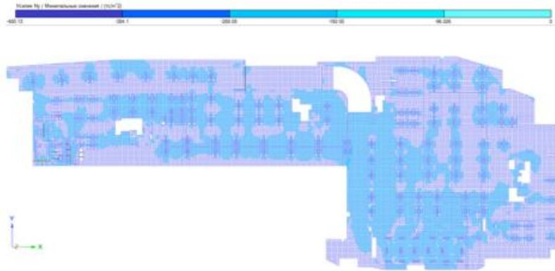
**Fig. 8.** Maximum values of  $N_y$  forces in the floor slab of the -2nd underground floor at -6,200.
