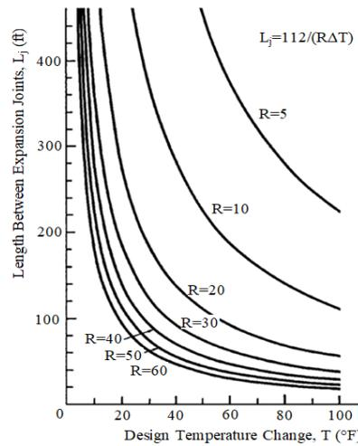
**Fig. 2.** Length between expansion joints versus design temperature change, AT (Martin & Acosta 1970)
