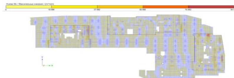
**Fig. 13.** Maximum values of forces  $M_x$  in the floor slab -1st underground floor at the level -0,900.
