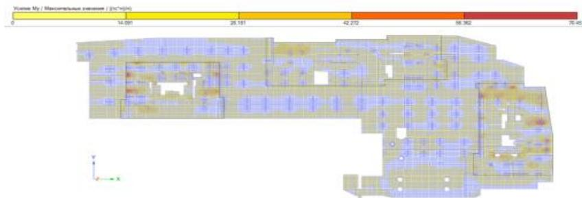
**Fig. 14.** Maximum values of  $M_y$  forces in the floor slab -1st underground floor at -0.900.
