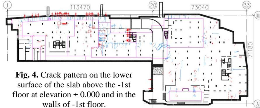
**Fig. 4.** Crack pattern on the lower surface of the slab above the -1st floor at elevation  $\pm 0.000$  and in the walls of -1st floor.
