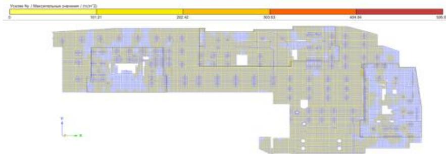
**Fig. 12.** Maximum values of  $N_y$  forces in the floor slab -1st underground floor at -0,900.
