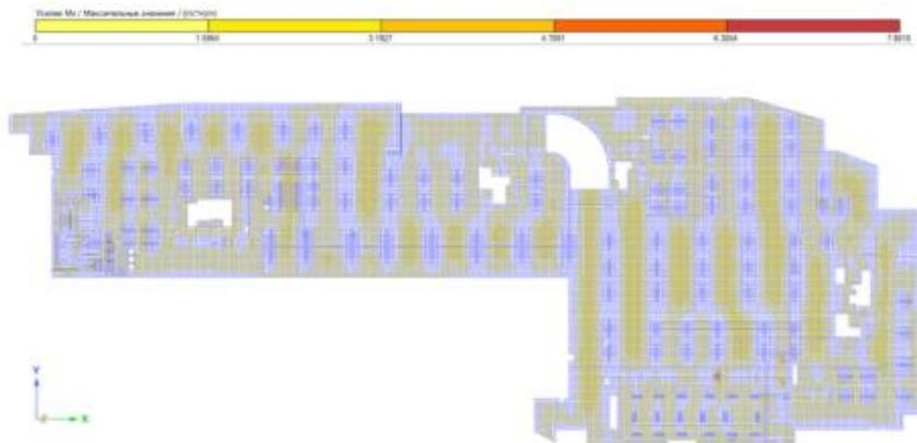
**Fig. 9.** Maximum values of  $M_x$  forces in the floor slab of the -2nd underground floor at -6,200.
