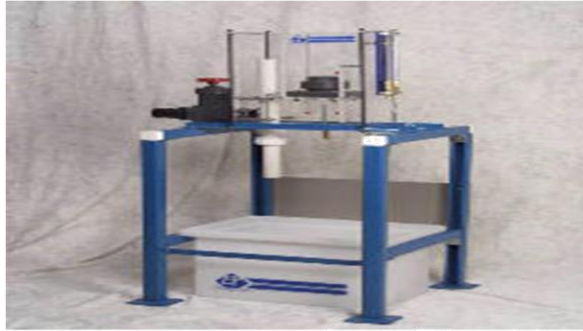
Figure 8 Constant head testing with Geo-Textile placed in the Sample chamber
