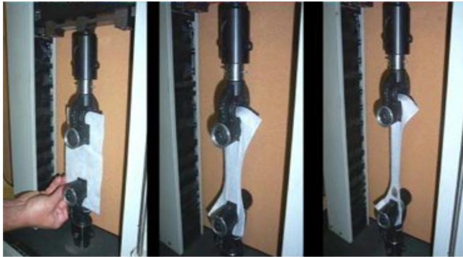
Figure 6: Checking Tensile Strength (As it can be seen that first sample placed between two grips. Then load is applied at constant rate till the Geo-Textile sample gets raptured)
