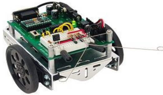
Fig 1. Real system differential structure of a mobile robot.
