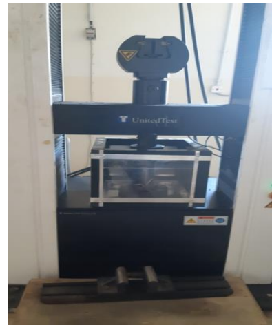
Figure 3. Compression Test apparatus with the tool of hydroforming
