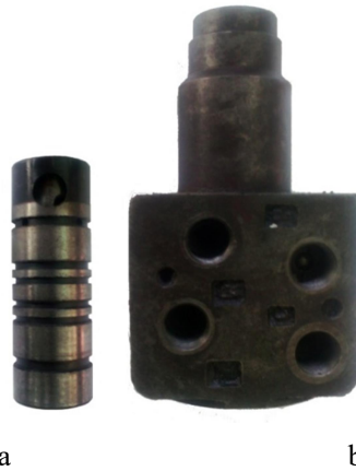
Fig. 1: Slide valve (a) and housing of hydraulic steer (b).
