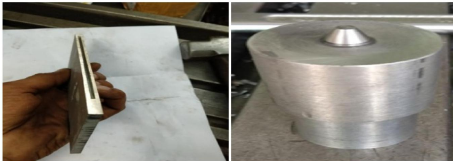
Fig.1.a: Grooves prepared at joint interface for particle reinforcement b. (f) tool used
