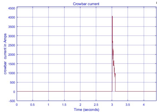
Fig. 13: Crowbar current during voltage dip
