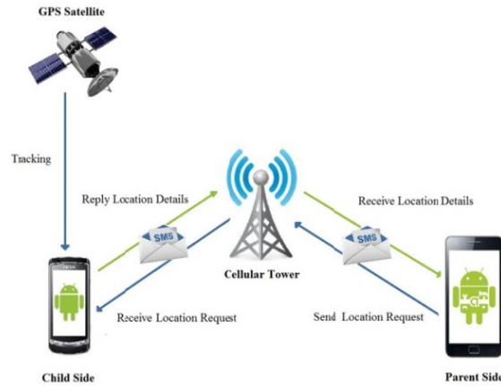
Fig. 4: Child tracking architecture using GPS
