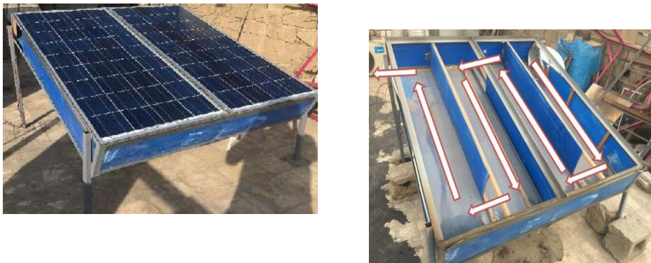
Figure (4) Solar panels setup and air ducts passages.
