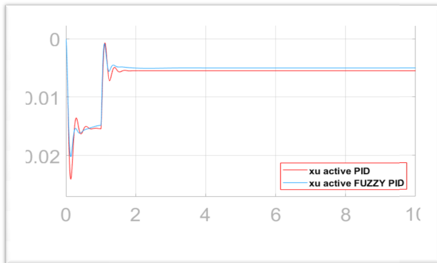
Fig. (15): Unsprung Mass displacement for active FUZZY PID and PID control
