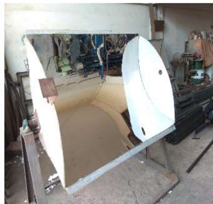
Fig 3. Parabola with reflective sheet
