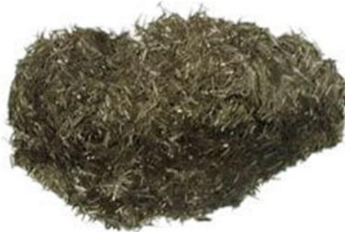
Fig. 5: Basalt Fiber Chopped Strands
