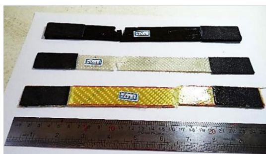
Fig. 2: Tensile test specimens with tab of sandpaper
