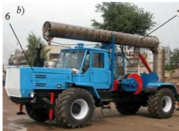
Fig. 1: Machines for the implementation of foundations in rammed pits
