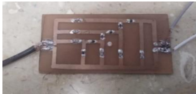
Figure 5. Developed Dickson type three stages Voltage multiplier circuit (Prototype-2)
